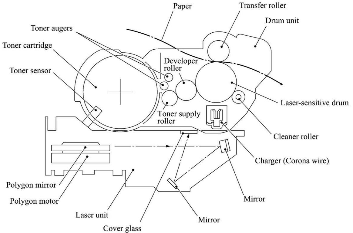
The print process unit works with laser beam, electrical charges, and toner. The graph below shows the transition of electrical charge on the surface of the laser-sensitive drum through the five processes: charging, exposing, developing, transferring, and erasing processes.
