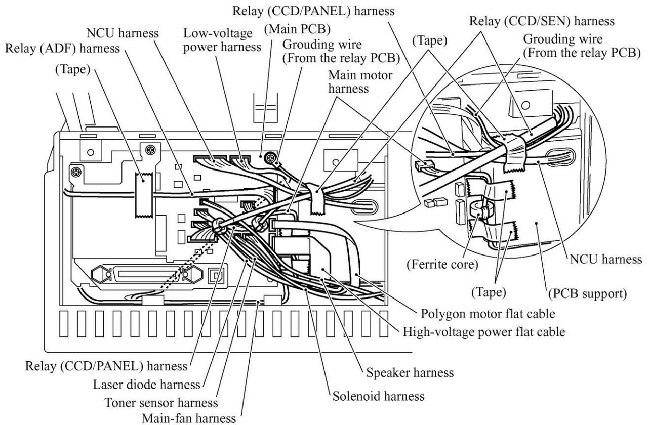
**Harness routing E: Relay harnesses on the main cover (after the ASF is removed)**
