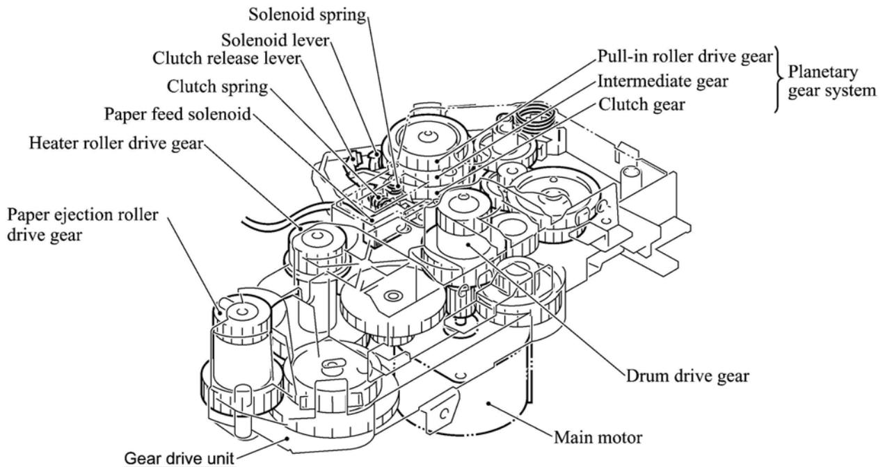
The paper pulling-in and registration mechanism consists of the pull-in roller gear (incorporated in the auto sheet feeder ASF), planetary gear system, paper feed solenoid, solenoid lever, clutch release lever, and registration sensor. (For the details about the sensor, refer to Subsection 3.2.3.)
