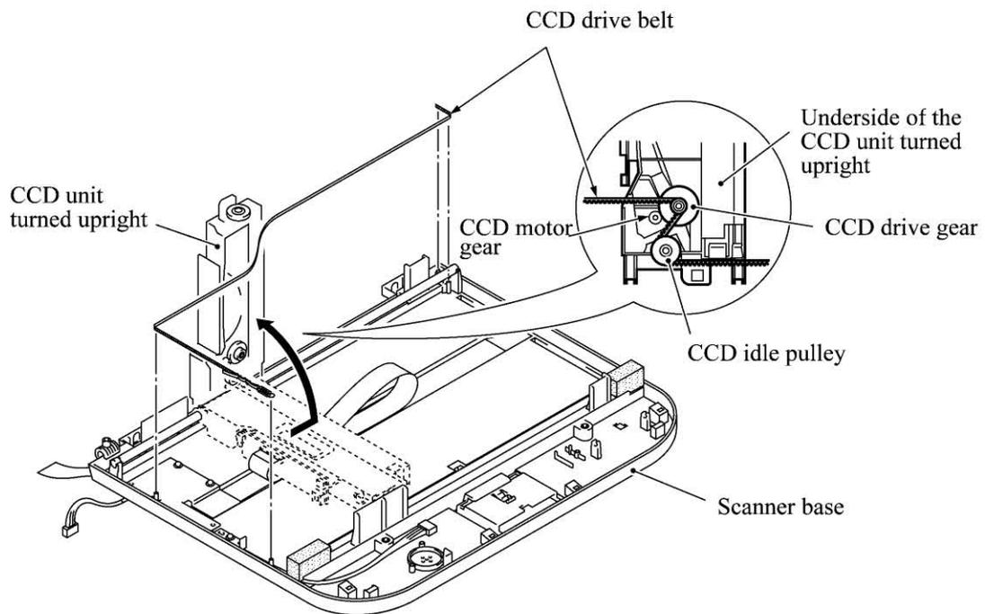
The CCD unit contains a charge coupled device (CCD) image sensor. The cold-cathode fluorescent lamp illuminates a document and the reflected light of the scanned image data is transmitted via the mirrors into the lens which reduces the scanned data so as to form the image on the CCD.
