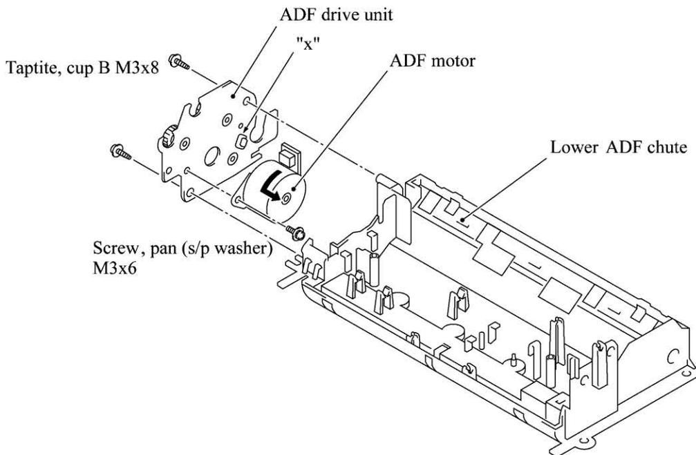
**Reassembling Note:** When setting the ADF motor, hook the non-screw side of the flange on section "x" (shown above) and secure it with the screw.
