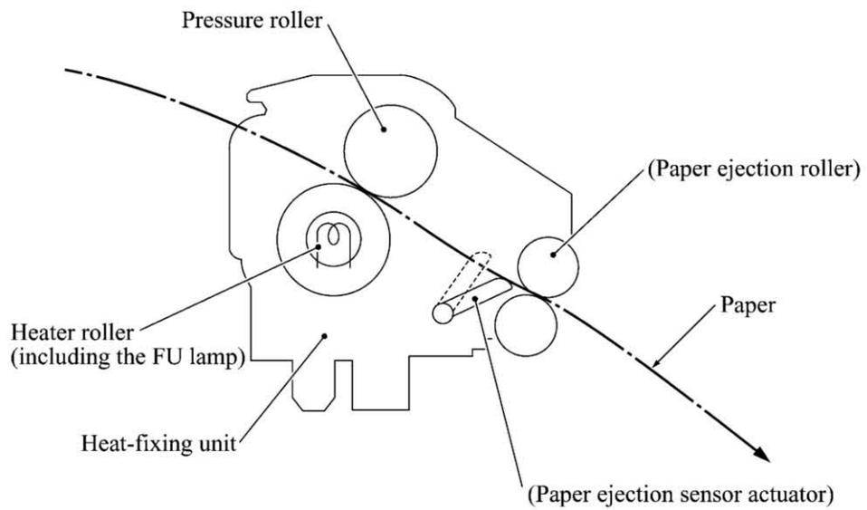
As the paper passes between the heater roller and the pressure roller in the heat-fixing unit, the heater roller fuses the toner on the paper.
