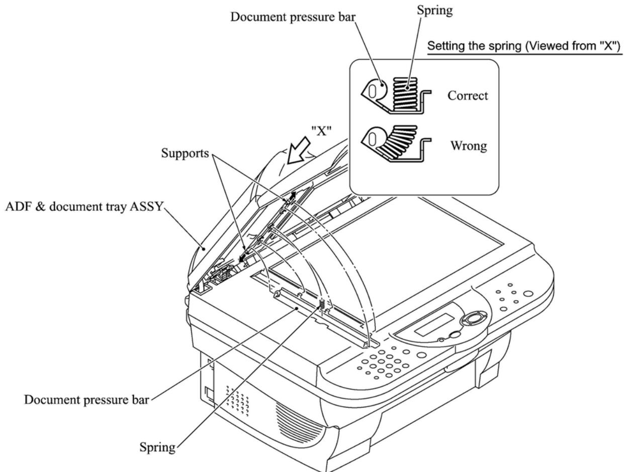
**Reassembling Note:** After setting the document pressure bar, check in the direction of arrow "X" that the spring is into place as illustrated above.
