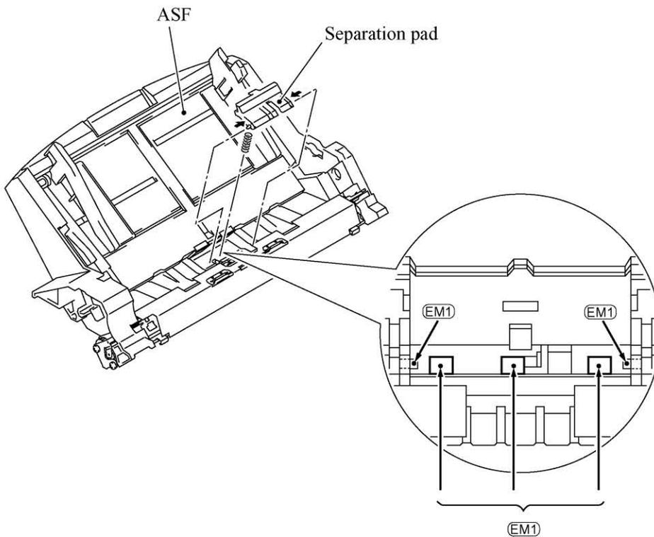
(Apply thin coat of grease to these sections with a brush where the separation pad is to be mounted.)
