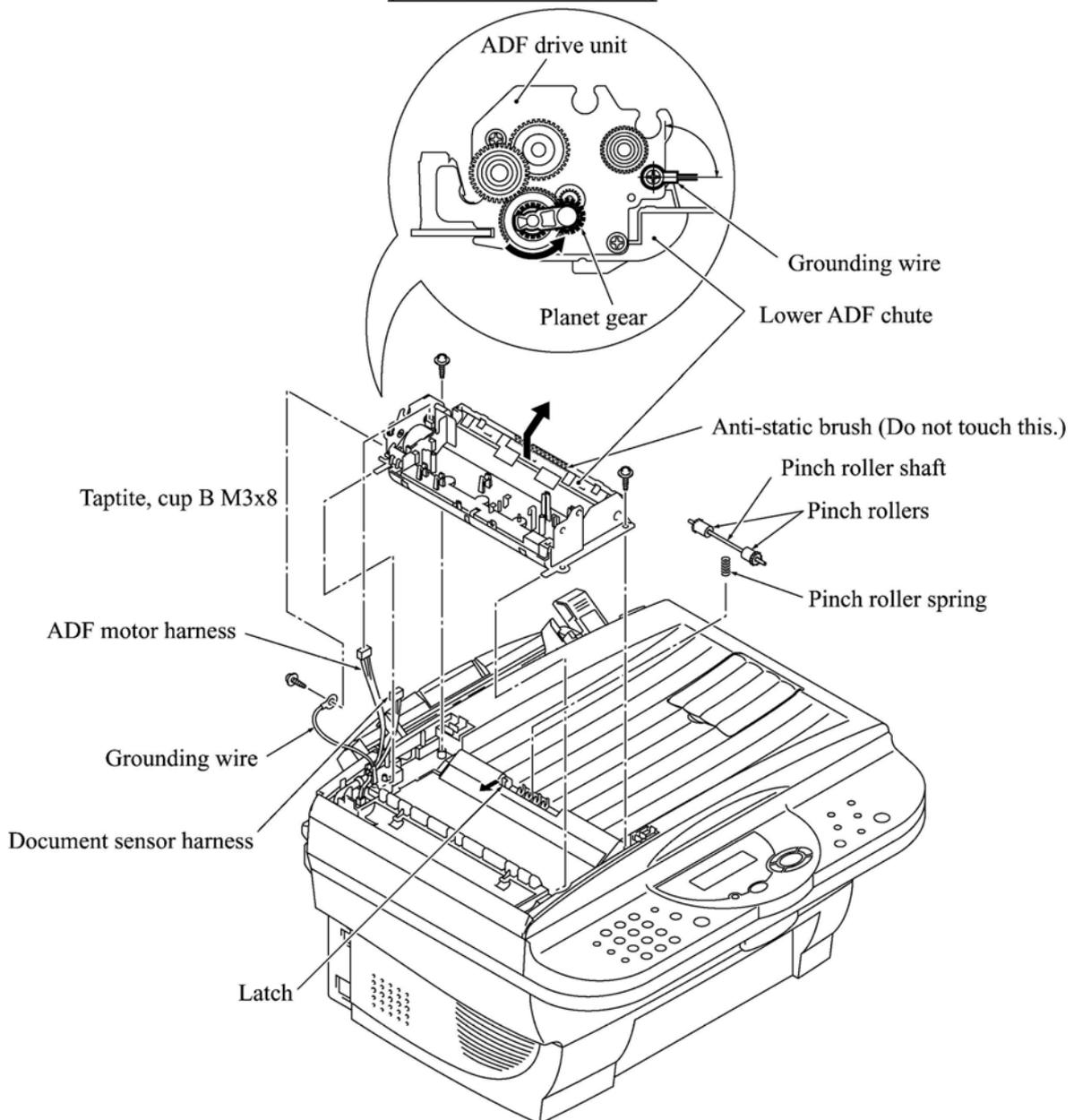
(15) Remove the two screws from the ADF drive unit and release the ADF motor.
