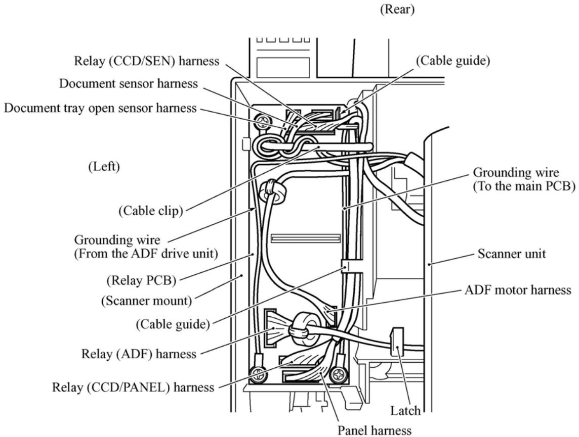
**Harness routing C: Relay (ADF) harness on the scanner mount**
