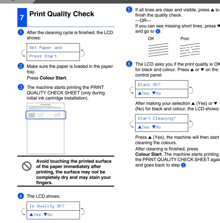
Check the quality of the four colour blocks formed by the short lines printed on the sheet. (BLACK/ CYAN/ YELLOW/ MAGENTA)
