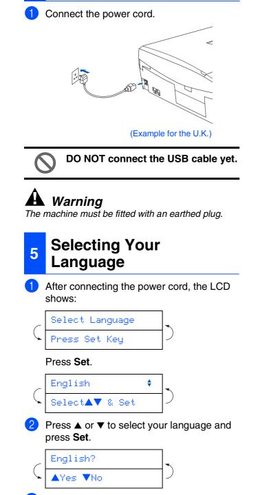
**Installing the Power**
