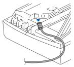
3. Carefully guide the network cable into the trench as shown below, following the trench round and toward the back of the machine.
