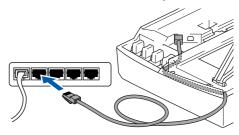
Make sure that the cable does not restrict the cover from closing, or an error may occur.
