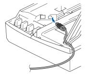
**12** Carefully route the USB cable through the trench and out the back of the machine as shown below.
