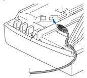
Second Carefully route the USB cable through the trench and out the back of the machine as shown below.
