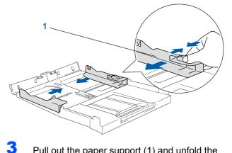
Pull out the paper support (1) and unfold the paper support flap (2).
