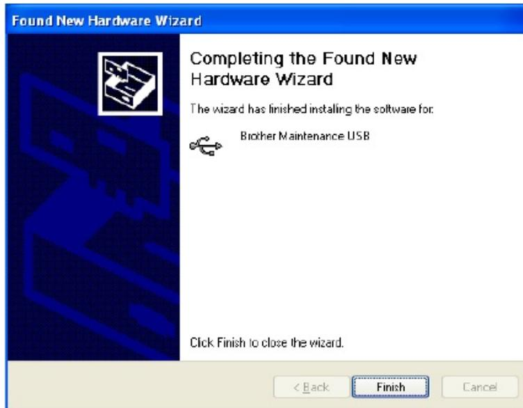
**NOTE:** In order to check whether the printer driver is successfully installed, click **Start | Settings | Printers** to select the Printers window. Then, check that the Brother Maintenance USB Printer icon is shown.
