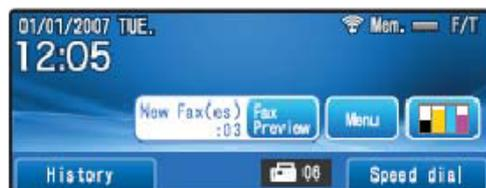
**TIP:** When the touch panel is inoperable, simultaneously press the **Scan** and **Copy** keys on the control panel, instead of the **Menu** key.
