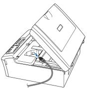
Carefully route the USB cable through the trench and out the back of the machine as shown below.
