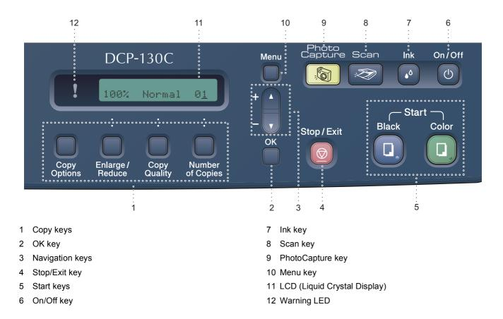
For the details of the control panel, see Control panel overview in Chapter 1 of the User's Guide.
