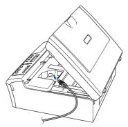
12 Carefully route the USB cable through the trench and out the back of the machine as shown below.
