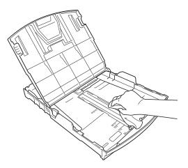
Close the output paper tray cover and put the paper tray firmly back in the machine.
