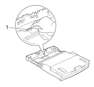
3 Open the Jam Clear Cover (1) at the back of the machine.
