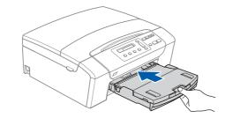
h. Pull out the paper support 1 until it clicks, and then unfold the paper support flap 2.
