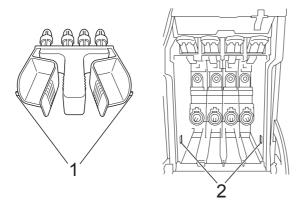
If you are not able to find the green protective part, DO NOT remove the ink cartridges before shipping. It is essential that the machine be shipped with either the green protective part or the ink cartridges in position. Shipping without them will cause damage to your machine and may void your warranty.
