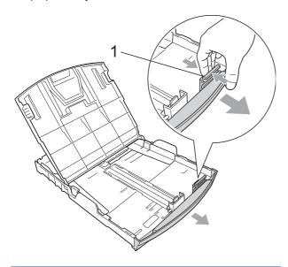
6 Gently adjust the paper side guides (1) to the paper with both hands. Make sure the paper side guides touch the sides of the paper.
