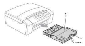
Pull out the jammed paper (1) and press Stop/Exit.
