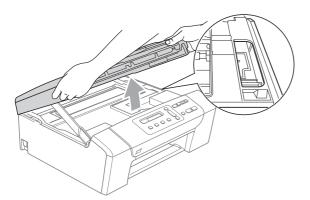
If ink gets on your skin or clothing immediately wash it off with soap or detergent. Lift the scanner cover to release the lock (1). Gently push the scanner cover support down (2) and close the scanner cover (3) using both hands.
