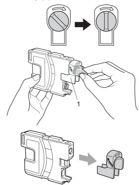
Each colour has its own correct position. Insert the ink cartridge in the direction of the arrow on the label.
