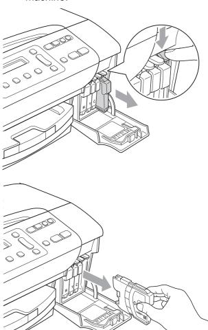
Open the new ink cartridge bag for the colour shown on the LCD, and then take out the ink cartridge.
