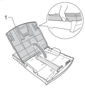
With both hands, gently press and slide the paper side guides (1) and paper length guide (2) to fit the paper size. Make sure that the triangular marks (3) on the paper side guides (1) and paper length guide (2) line up with the mark for the paper size you are using.
