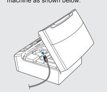
C. Carefully route the USB cable through the cable channel and out the back of the machine.
