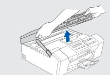
**b.** Connect the USB cable to the USB socket marked with a symbol. The USB socket is inside the machine as shown below.
