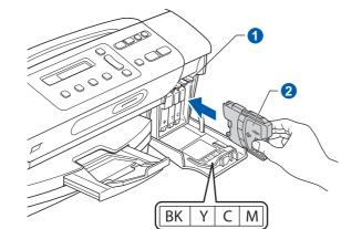
**f.** Gently push the ink cartridge until it clicks. After all the ink cartridges are installed close the ink cartridge cover.
