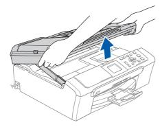
Insert the network cable into the LAN socket marked with a R symbol. You will find the LAN socket inside the machine on the left as shown below.
