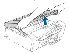
Insert the USB cable into the USB socket marked with a 🚭 symbol. You will find the USB socket inside the machine as shown below.
