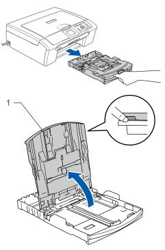
Press and slide the paper side guides (1) and paper length guide (2) to fit the paper size.
