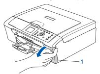
Pull all the lock release levers down and remove the yellow protective part (1).
