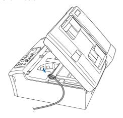
Carefully route the network cable through the trench and out the back of the machine as shown below.
