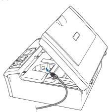
12 Carefully route the USB cable through the trench and out the back of the machine as shown below and connect the cable to your computer.
