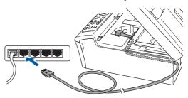
Make sure that the cable does not restrict the cover from closing, or an error may occur.
