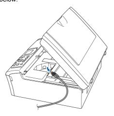
Carefully guide the USB cable into the trench as shown below, following the trench around and toward the back of the machine. Then, connect the cable to your Macintosh®.
