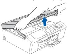
Connect the USB cable to the USB socket marked with a + symbol. You will find the USB socket inside the machine as shown below.
