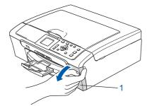
Pull all the lock release levers down and remove the yellow protective part (1).
