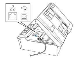
Carefully guide the network cable into the trench as shown below, following the trench around and toward the back of the machine. Then, connect the cable to your network.
