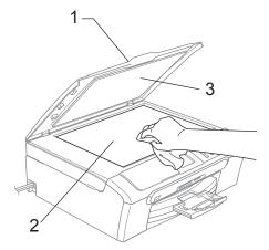
(DCP-560CN only) In the ADF unit, clean the white bar (1) and the glass strip (2) with a lint-free cloth moistened with a non-flammable glass cleaner.
