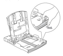
Gently adjust the paper side guides to the paper with both hands. Make sure the paper side guides touch the sides of the paper.
