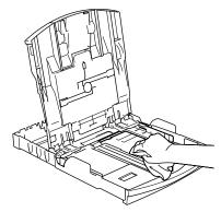
5 Close the output paper tray cover and put the paper tray firmly back in the machine.
