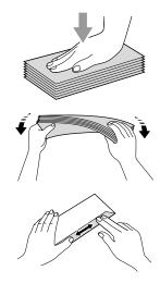
Put the envelopes or post cards into the paper tray with the address side down and the leading edge in first as shown in the illustration. Slide the paper side guides (1) and paper length guide (2) to fit the size of the envelopes or post cards.
