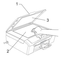
(DCP-560CN only) In the ADF unit, clean the white bar (1) and the glass strip (2) with a lint-free cloth moistened with a non-flammable glass cleaner.
