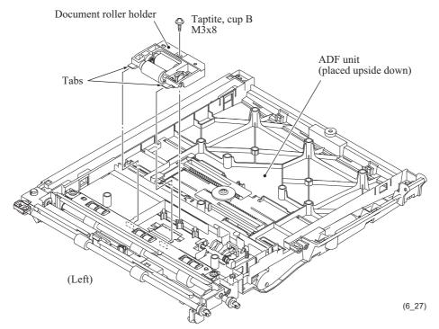
**Assembling Note:** Before mounting the document roller holder on the ADF unit, apply the specified lubricant to the specified points, referring to Section 6.2.
