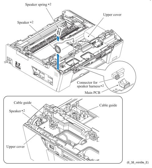
**Assembling Note:** After mounting the speaker  $^{*2}$  and its spring  $^{*2}$  into the pocket provided on the upper cover, route the speaker harness  $^{*2}$  through the cable guide on the upper cover as shown on the previous page.
