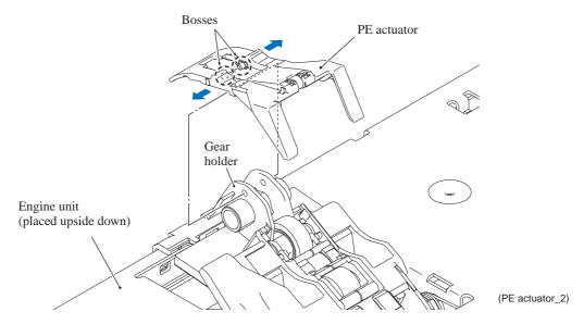
2) Lift up the front end of the PE actuator. After fitting the short end of the PE actuator spring into the groove provided in the gear holder, set the spring back into place, and then fit the long end into the groove in the PE actuator.
