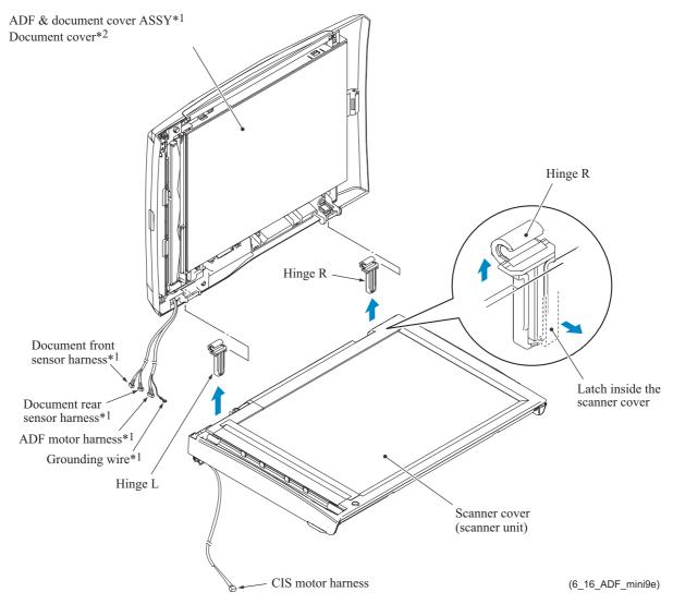
**Assembling Note:** When mounting the ADF & document cover ASSY\*1 on the scanner cover, put a magazine or a stack of paper about 2 to 3 cm (one inch) thick between them to secure room for looseness of harnesses. Do not use the one that may scratch or contaminate the scanner glass.
