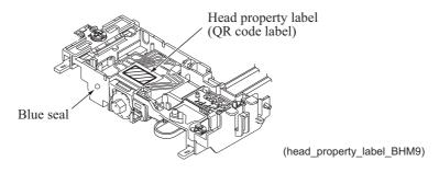
**Note:** Depending on whether the head/carriage unit has a round, blue seal on its left side, the purge type to be performed differs. Refer to Chapter 7, Section 7.2 [2].
