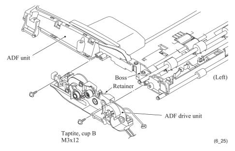
**Assembling Note:** When mounting the ADF drive unit on the ADF unit, route the ADF motor harness and its grounding wire and the document front sensor harness below the cable guides (see page 6-21).
