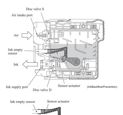
Attached to one end of the sensor actuator is a float. When there is ink in the cartridge, buoyancy lifts the float, rotating the sensor actuator about a pivot near the center of the actuator to block the light beam to the ink empty sensor, indicating that there is ink.
