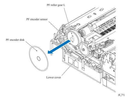
**Assembling Note:** When attaching the PF encoder disk to the PF roller gear L, using a spatular tool makes the job easier. Put on clean gloves to protect the disk surface from dust or fingerprints.
