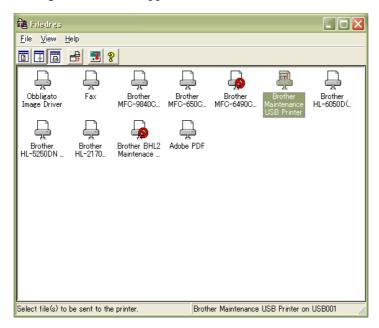
(4) Drag and drop the firmware (e.g., LZ0023\_A.pmu) onto the Brother Maintenance USB Printer driver icon in the Filedrgs window.
