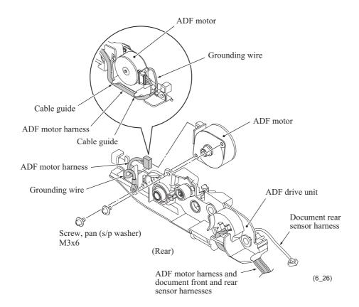
**Assembling Note:** When securing the ADF motor to the ADF drive unit with two screws, be sure to secure the grounding wire also with one of those screws. (See the illustration above.)
