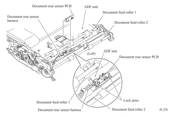
**Assembling Note:** Route the document rear sensor harness through the cable guides provided on the ADF unit as shown below.
