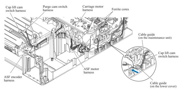
Note: When routing the cap lift cam switch harness on the lower cover, pass it under the 3rd cable guide counted from the rear without any slack, pulling it with your fingers.
