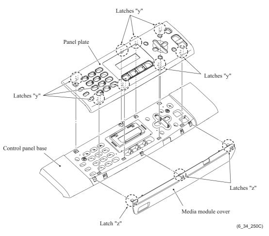
**Assembling Note:** Assemble the panel plate and the control panel base, taking care not to apply pressure to the media module cover.
