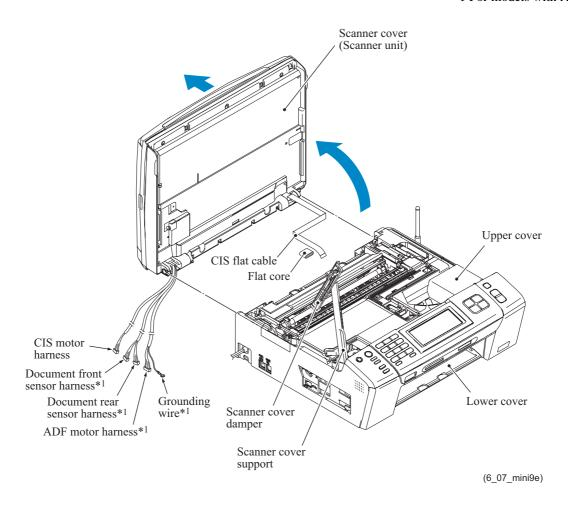
**Assembling Note:** If you replace the scanner cover, specify the CIS type into the EEPROM in the maintenance mode (Function code 59), referring to Chapter 9, Section 9.4.17. After that, acquire the white level data and set the CIS scanner area in the maintenance mode (Function code 55), referring to Chapter 9, Section 9.4.15.
