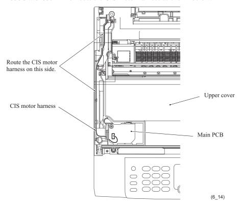
**Models with ADF:** Route the document front and rear sensor harnesses, CIS motor harness, ADF motor harness and grounding wire as shown below.
