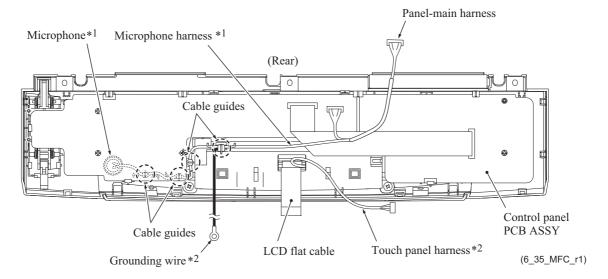
• After completion of assembling of the control panel ASSY, wipe fingerprints or dust off the LCD surface with a soft cloth.
