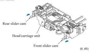
• When mounting the head/carriage unit on the left end of the engine unit, first fit the front end over the CR support chassis (shown on the previous page) and then set the rear end onto the CR guide rail. Make sure that the two front bosses (see below) provided on the bottom of the head/carriage unit catch the front edge of the CR support chassis and the two rear bosses are fitted in the two cutouts (shown on the previous page) in the CR guide rail.
