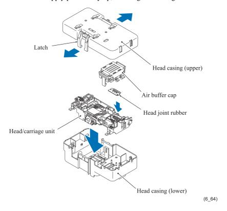
**Assembling Note:** After replacement of the head/carriage unit, make adjustments specified in Chapter 7, Section 7.2. (For the head/carriage unit having a round, blue seal, perform the head replacement purge; for the unit having no seal, perform the initial purge. See Section 7.2, [2].)
