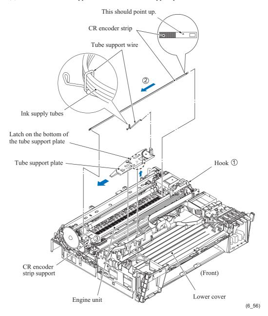
**Assembling Note:** After mounting the head cover, set the CR encoder strip so that the ▲-marked end is to the right (carriage motor side) and the mark points upwards as shown above, using the following steps.
