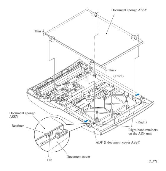
**Assembling Note:** When mounting the document sponge ASSY, orient it so that the thin end faces to the left. First insert the left front tab into the retainer provided on the ADF unit and then insert the left rear tab while warping the document sponge ASSY. Next push down the right side of the document sponge ASSY into place.
