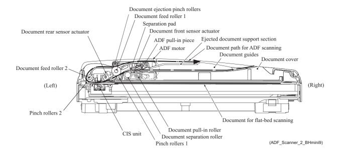
Models with ADF offer two types of scanning: ADF scanning and flat-bed scanning. They automatically switch to the former at the start of a scan operation if the document front sensor inside the ADF detects a document. Models without ADF offer only flat-bed scanning.
