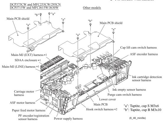
**Assembling Notes:** Before securing the main PCB shield, route the harnesses on the top of the lower cover as shown below. Make sure that the main-MJ (EXT) harness\*1 and main-MJ (LINE) harness\*1 are routed through the SDAA enclosure\*1. (See the illustration given on page 6-51 for the routing of those harnesses on the left side of the lower cover.)
