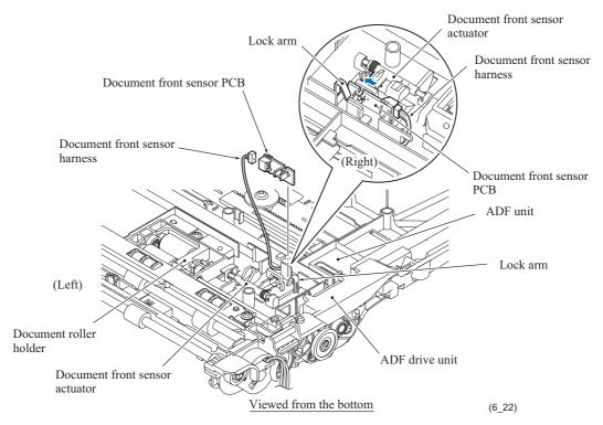
**Assembling Note:** Route the document front sensor harness through the cable guides provided on the ADF unit as shown below. Also route the ADF motor harness through the cable guides together with the document front sensor harness.
