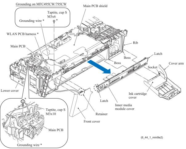
Grounding on DCP375CW/J315W/J515W/J715W and MFC255CW/J265W/J270W/J410W/J415W/J615W/J630W
