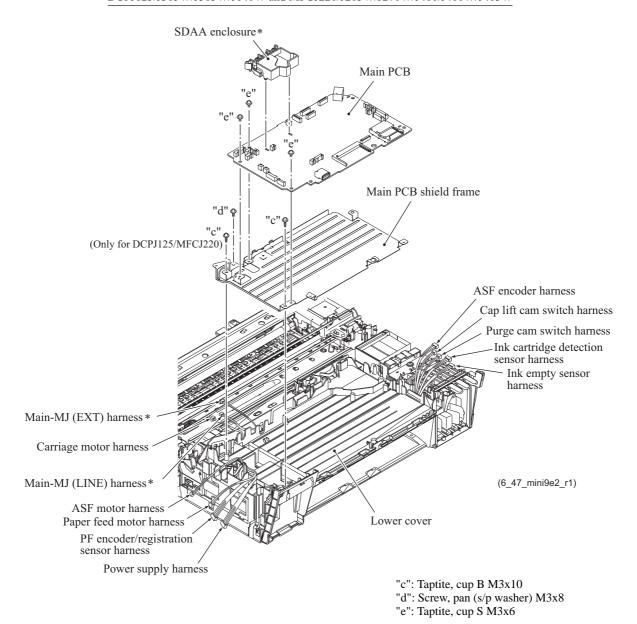
**Assembling Note:** If you replace the main PCB, you need to load programs onto the flash ROM, restore the machine information that has been backed up in an external memory (refer to Chapter 9, Section 9.4.11), and make specified adjustments of various settings (refer to Chapter 7, Section 7.3). Make sure beforehand that the head/carriage unit is mounted.
