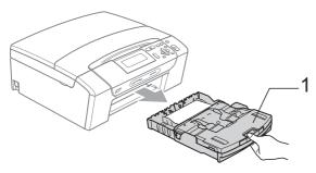
2 Pull out the jammed paper (1) and press **Stop/Exit**.
