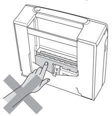
When moving the machine you must lift it from the base, by placing a hand at each side of the unit as shown in the illustration. DO NOT carry the machine by holding the scanner cover or the Jam Clear Cover.
