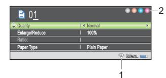
1 Wireless Status (DCP-585CW only) A four level indicator shows the current wireless signal strength if you are using a wireless connection.
