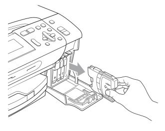
3 Open the new ink cartridge bag for the color shown on the LCD, and then take out the ink cartridge.
