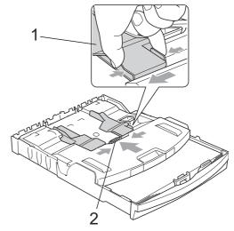
Put the photo paper into the photo bypass tray and gently adjust the paper side guides to the paper.
