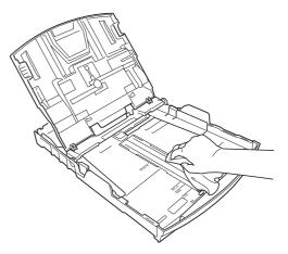
5 Close the output paper tray cover and put the paper tray firmly back in the machine.
