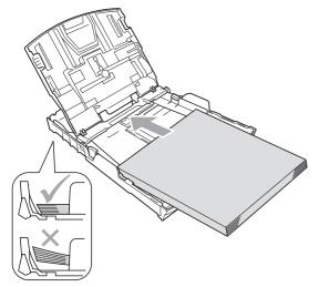
6 Gently adjust the paper side guides (1) to fit the paper with both hands. Make sure the paper side guides touch the sides of the paper.
