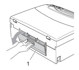
Clean the paper pick-up roller (1) with isopropyl alcohol on a cotton swab.
