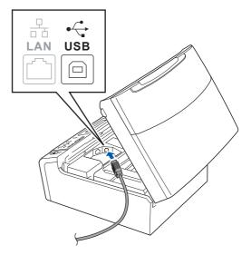
Carefully route the USB cable through the trench and out the back of the machine as shown below and connect the cable to your Macintosh.
