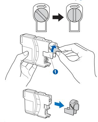
Take care to match the color of the lever 1 with the cartridge color 2, as shown in the diagram below.
