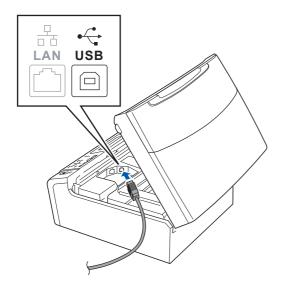
Carefully route the USB cable through the trench and out the back of the machine as shown below and connect the cable to your computer.
