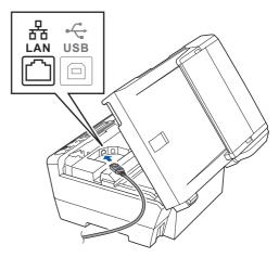
Carefully guide the network cable to the trench as shown below, following the trench around and toward the back of the machine. Then, connect the cable to your network.
