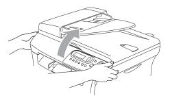
You can still use the machine when the scanner cover is raised. You can return the scanner cover to its home position by pushing it down with both hands.
