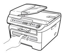
Using both hands, slide the manual feed slot paper guides to the width of the paper that you are going to use.
