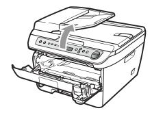
Use both hands to carefully pull the jammed paper up and out of the output tray opening.
