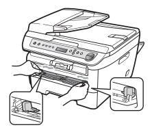
4 Using both hands, put one sheet of paper or one envelope in the manual feed slot until the front edge of the paper or envelope touches the paper feed roller. When you feel the machine pull in the paper, let go.
