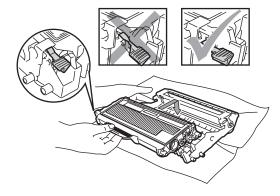
9 Put the drum unit and toner cartridge assembly back in the machine.
