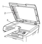
(DCP-7040 and DCP-7045N) In the ADF unit, clean the white bar (1) and the scanner glass strip (2) underneath it with a soft lint-free cloth moistened with water.
