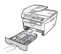
While pressing the green paper guide release lever, slide the paper guides to fit the paper size. Make sure that the guides are firmly in the slots.
