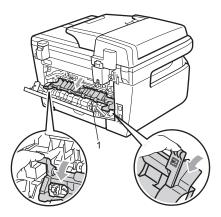
5 Pull the jammed paper out of the fuser unit.
