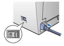
2 Plug the AC power cord into an AC outlet. Turn the power switch on.
