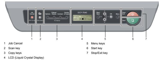
For the details of the control panel, see Control panel overview in Chapter 1 of the User's Guide.
