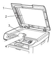
(DCP-7040 only) In the ADF unit, clean the white bar (1) and the scanner glass strip (2) underneath it with a soft lint-free cloth moistened with water.
