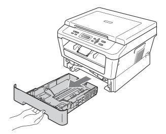
**b** While pressing the green paper-guide release lever (1), slide the paper guides to fit the paper size you are loading in the tray. Make sure that the guides are firmly in the slots.
