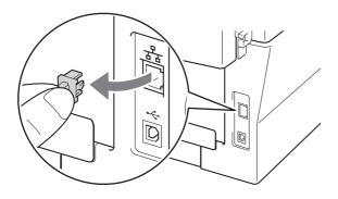
С Connect the network interface cable to the LAN connector and then connect it to a free port on your hub.
