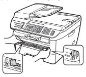
4 Using both hands, put one sheet of paper or one transparency in the manual feed slot until the front edge touches the paper feed roller. When you feel the machine pull in the paper, let go.
