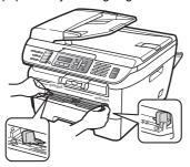
Using both hands, put one sheet of paper or one envelope in the manual feed slot until the front edge of the paper or envelope touches the paper feed roller. When you feel the machine pull in the paper, let go.
