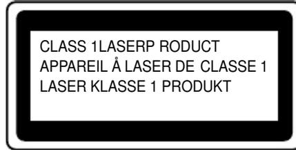
This printer has a laser diode which emits invisible laser radiation in the Laser Unit. The Laser Unit should not be opened without disconnecting the two connectors connected with the AC power supply and laser unit. Since the variable resistor in the laser unit is adjusted in accordance with the standards, never touch it.
