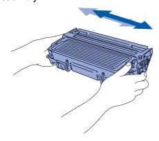
4 Push the drum unit assembly into the DCP (until it snaps into place).
