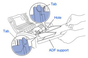
3 Push ADF Support down until it latches in place.
