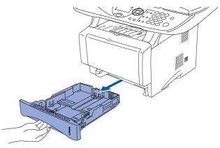
While pressing the paper guide release lever, slide the adjusters to fit the paper size. Check that the guides are firmly in the slots on the tray.
