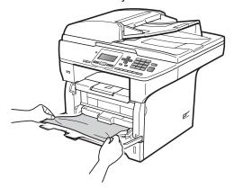
Close the MP tray. Then open the front cover and close it to reset the machine. Open the MP tray again.
