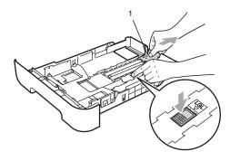
4 Put paper in the tray, and make sure that the paper is below the maximum paper mark (1). The side to be printed on must be face down.
