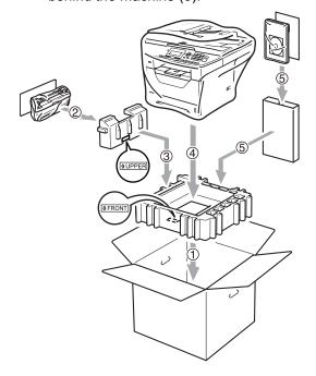
Put the two styrofoam pieces into the carton matching. Match the front of the machine to the "FRONT" mark on one of the styrofoam pieces, and the back of the machine to the "REAR" mark on the other styrofoam piece (6). Put the AC power cord and printed materials in the original carton as shown below (7).
