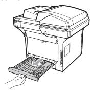
Pull the jammed paper out of the machine or the duplex tray.
