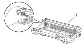
6 When you have found the mark on the drum that matches the print sample, wipe the surface of the OPC drum with a dry cotton swab until the dust or glue on the surface comes off.
