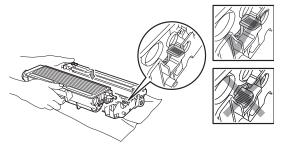
8 Put the drum unit and toner cartridge assembly back in the machine.
