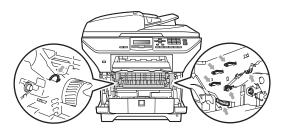
5 Put the drum unit and toner cartridge assembly back in the machine.
