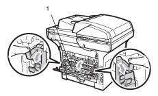
5 Pull the jammed paper out of the fuser unit.
