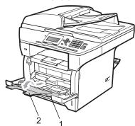
While pressing the paper side guide release lever, slide the paper guides to fit the width of the paper that you are going to use.
