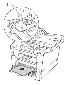
4 Lift up the support flap to prevent paper from sliding off the face-down output tray, or remove each page as soon as it comes out of the machine.
