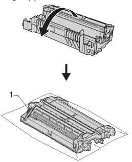
8 Use the numbered markers next to the drum roller to find the mark. For example, a dot in column 2 on the check sheet would mean that there is a mark in the "2" region of the drum.
