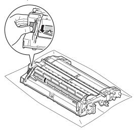
When you have found the mark on the drum that matches the drum dot check sheet, wipe the surface of the drum gently with a dry cotton swab until the mark on the surface comes off.
