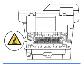
Using both hands, gently pull the jammed paper out of the back of the machine.
