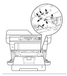
6 Push down the green lock lever and take the toner cartridge out of the drum unit. Remove the jammed paper if there is any inside the drum unit.
