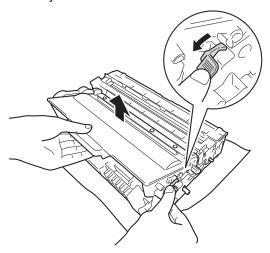
Put the toner cartridge back into the drum unit until you hear it lock into place. If you have put the cartridge in correctly, the green lock lever will lift automatically.
