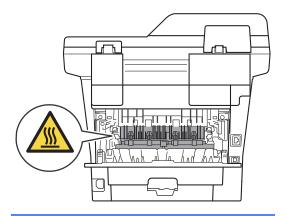
5 Pull the green tabs at the left and right hand sides toward you and fold down the fuser cover (1).
