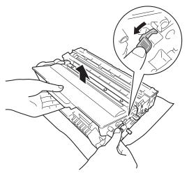
7 Turn the drum unit as shown in the illustration. Make sure that the drum unit gear (1) is on the left hand side.
