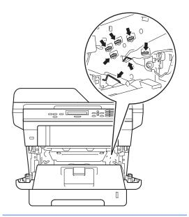
4 Clean the corona wire inside the drum unit by gently sliding the green tab back and forth several times.
