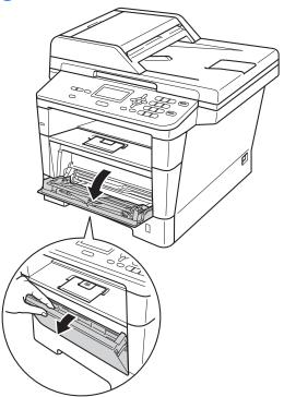
Pull out the MP tray support (1) and unfold the flap (2).
