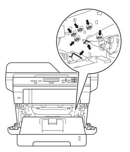
6 Push down the green lock lever and take the toner cartridge out of the drum unit.
