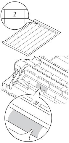
9 Turn the drum unit gear toward you by hand while checking the surface of the suspected area.
