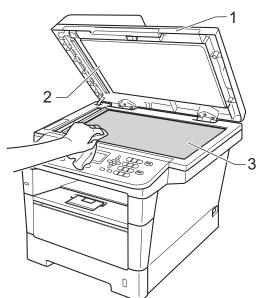
In the ADF unit, clean the white bar (1) and the scanner glass strip (2) underneath it with a soft lint-free cloth moistened with water.
