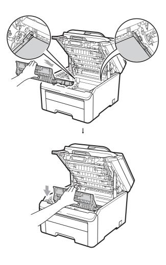
6 Slide each drum unit and toner cartridge assembly into the machine. Make sure that you match the toner cartridge colour to the same colour label on the machine. Repeat this for all the drum unit and toner cartridge assemblies.
