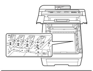
4 Push down the green-labelled lock lever (1) and take the toner cartridge out of the drum unit.
