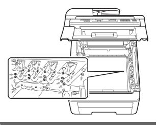
4 Clean the primary corona wire inside the drum unit by gently sliding the green tab from left to right and right to left several times.
