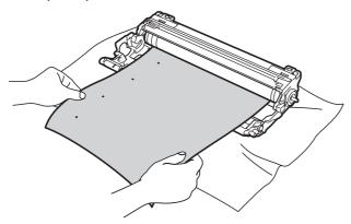
Turn the drum unit gear by hand while looking at the surface of the OPC drum (1).
