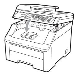
When the top cover is open, you cannot open the scanner.
