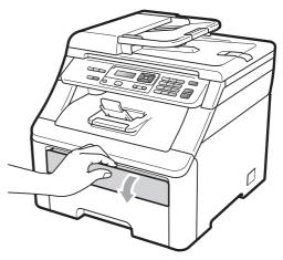
3 Using both hands, slide the manual feed slot paper guides to the width of the paper that you are going to use.
