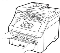
4 Using both hands, put one piece of paper in the manual feed slot with the print side face up until the front edge of the paper touches the paper feed roller. Wait until the machine automatically feeds the paper. When you feel the machine pull in the paper, let go.
