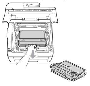
8 Reinstall the belt unit back in the machine.
