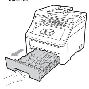
While pressing the green paper-guide release lever (1), slide the paper guides to fit the paper size you are loading in the tray. Make sure that the guides are firmly in the slots.
