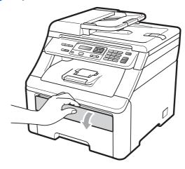
2 Using both hands, slide the manual feed slot paper guides to the width of the paper that you are going to use.
