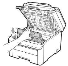
9 Reinstall the original packing material into the machine.
