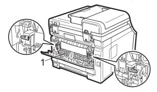
Using both hands, gently pull the jammed paper out of the fuser unit.
