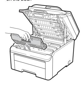
4 Push down the green-labelled lock lever (1) and take the toner cartridge out of the drum unit.
