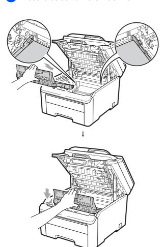
Slide each drum unit and toner cartridge assembly into the machine. Make sure that you match the toner cartridge colour to the same colour label on the machine. Repeat this for all the drum unit and toner cartridge assemblies.
