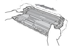
Slide all four drum and toner cartridge assemblies into the machine. Make sure the toner cartridge colour matches the same colour label on the machine.
