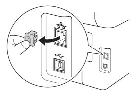
Connect the network interface cable to the Ethernet port on your machine, and then connect it to a free port on your hub.
