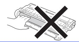
Remove the orange packing piece from the belt
