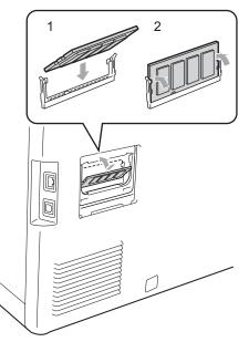
6 Put the metal (2) and then the plastic (1) SO-DIMM covers back on.
