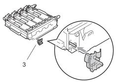
10 Put a piece of paper (A4 or Letter) on the belt unit to prevent damage to the belt unit.
