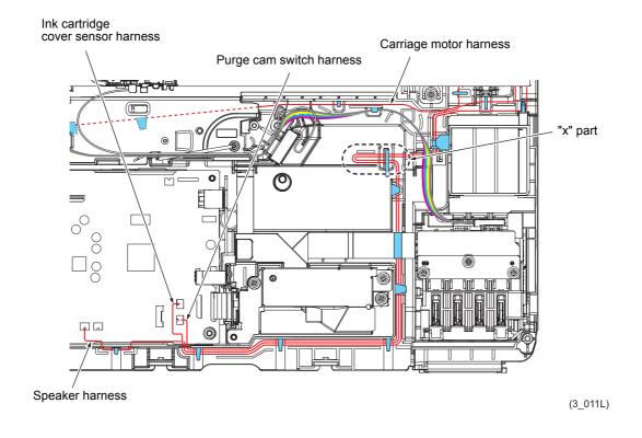
**Note** Bend the Purge cam switch harness and Speaker harness in "x" as shown above.
