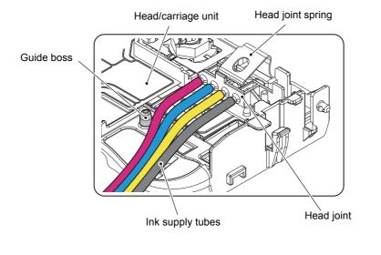
**Note** Make sure that all of the four lnk supply tubes are routed in front of the guide boss as shown above.
