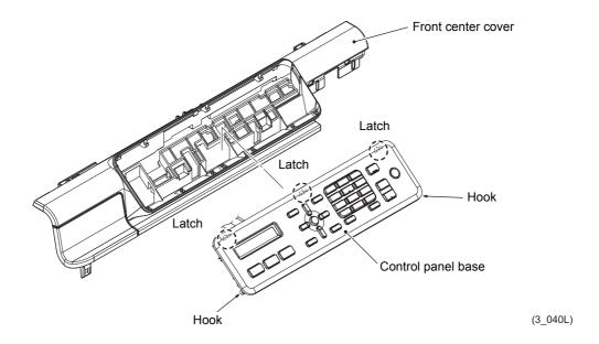
(6) Release the two latches and two hooks of the Printed panel cover, and remove the Panel PCB ASSY.
