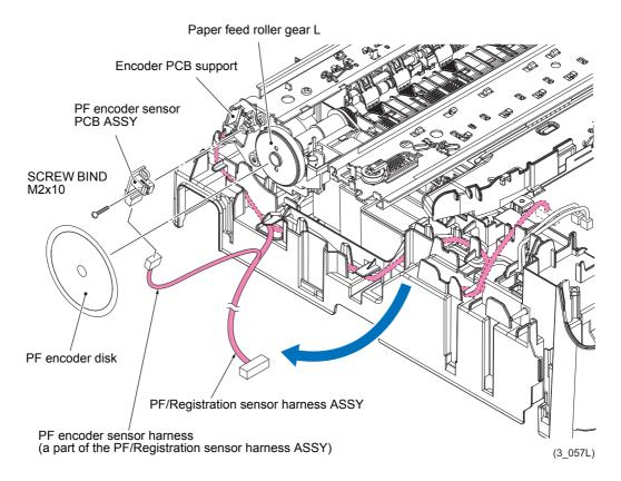
**Assembling Note** It is more convenient to use a spatula when attaching the PF encoder disk to the Paper feed roller gear L. Wear clean gloves to protect the disk surface from dust or fingerprints.
