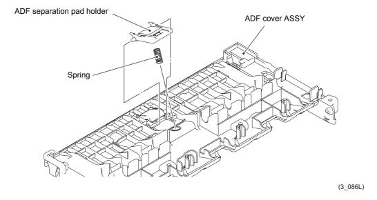
Assembling Note Insert the spring first into the opening then attach the ADF separation pad holder.
