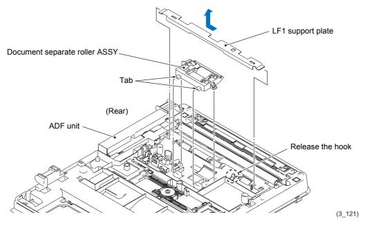
**Assembling Note** Before installing the Document separate roller ASSY to the ADF unit, refer to Section 5 in this chapter and apply the specified lubricant to all roller shafts.
