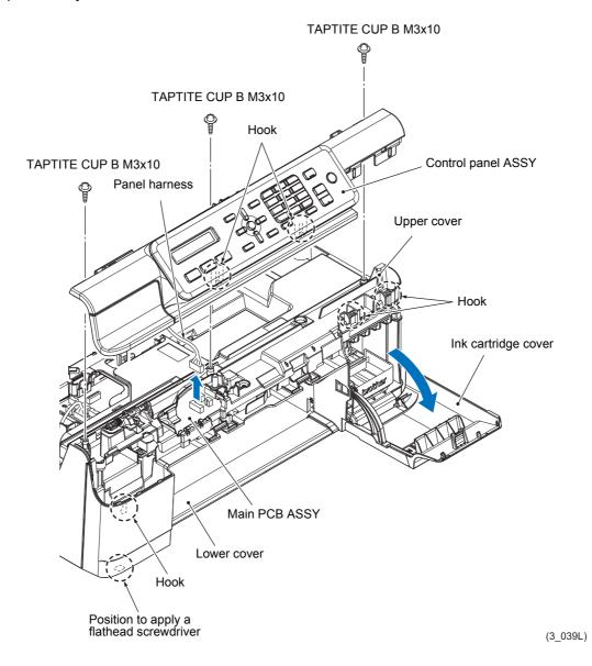
**Assembling Note** After installing the control panel ASSY in the upper cover, confirm that there is no gap between the front ends of the control panel ASSY and the upper cover.
