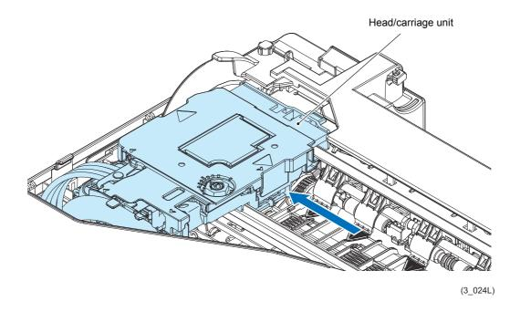
(9) Release the four latches with the ▲ mark on the Head cover, and then remove the Head cover.
