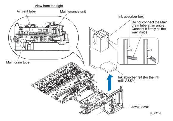
(3) Take the lnk absorber felt (for the lnk refill ASSY) out of the Lower cover.
