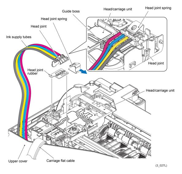
**Assembling Note** Make sure that all of the four lnk supply tubes are routed in front of the guide boss as shown above.
