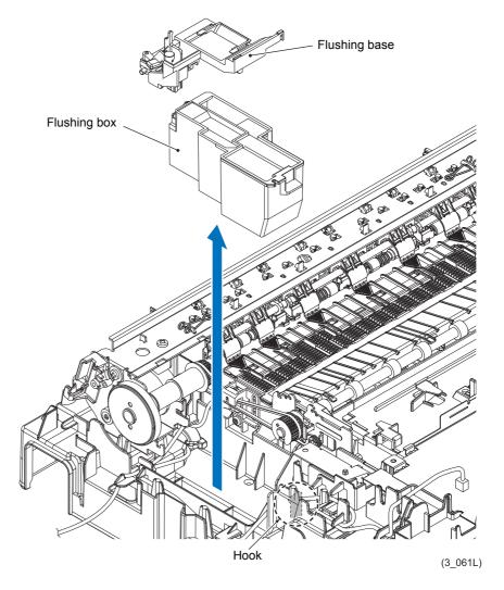
**Assembling Note** When the Flushing box is replaced (without replacement of the Main PCB ASSY), reset the flushing count as described in Chapter 4 "1.12 Reset Purge and Flushing Counts (Maintenance mode 80)".
