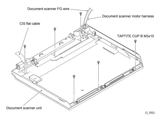
**Assembling Note** When mounting the Document scanner top cover, tighten the screws in the following order.
