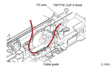
**Assembling Note** Route the FG wire along the cable guide (marked by the dotted circle) as shown above.
