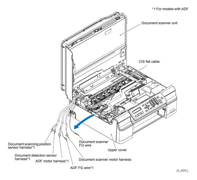
**Assembling Note** Route the Document scanning position sensor harness and Document detection sensor harness, and then route the Document scanner FG wire, Document scanner motor harness, ADF motor harness\*1, and ADF FG wire\*1. (Refer to the figure in Section 7-1 of this chapter)
