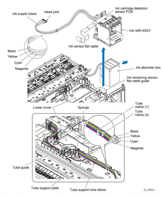
**Note** • Do not remove the Protective part. Doing so in this state will make the ink inside the ink tubes flow out.
