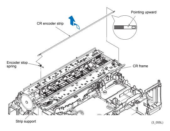
**Assembling Note** Attach the CR encoder strip with the end with the ▲ mark on the right (Carriage motor side) and the ▲ mark facing upward. (Refer to the illustration above)
