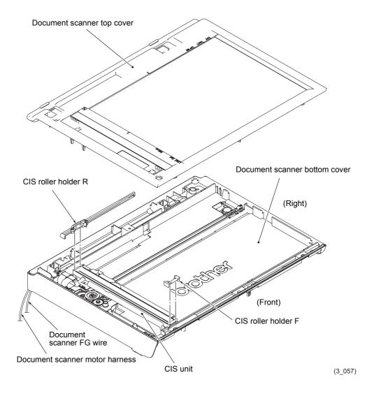
**Assembling Note** When attaching the CIS roller holder R, fit the projection into the lower side of the CIS unit.
