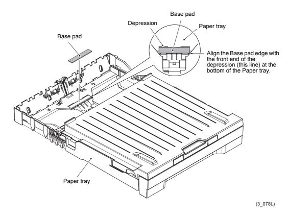
**Assembling Note** When attaching a new Base pad to the Paper tray, align the front end of the pad with the front end of the depression, and the left and right position with the center of the depression, as shown above.
