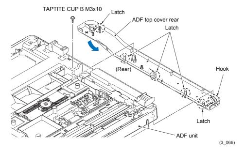
**Assembling Note** When mounting the ADF top cover rear, fit the hook first before pushing the cover in place.
