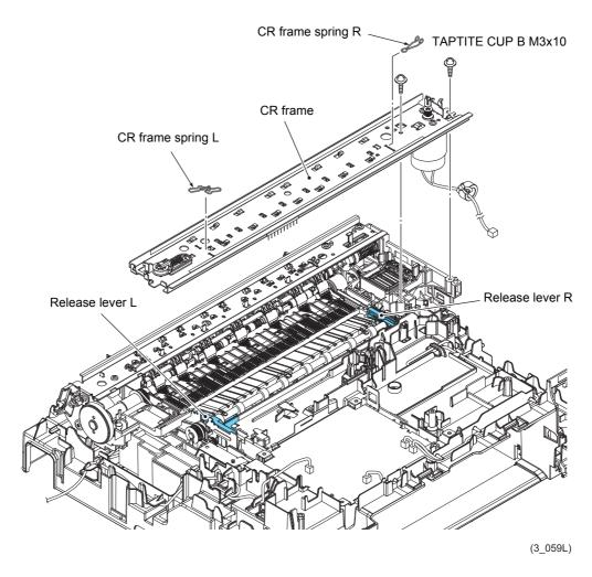
**Assembling Note** Make sure that the Release levers L/R are on your side.
