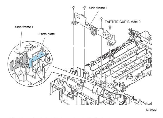
**Assembling Note** Attach the Side frame L under the Earth plate.
