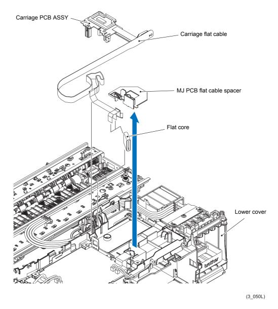
**Note** When replacing the Carriage PCB ASSY, remove the Flat core from the old cable and attach it to the new cable.
