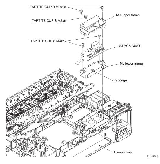
**Assembling Note** When installing the MJ PCB, make sure that the sponge is attached.
