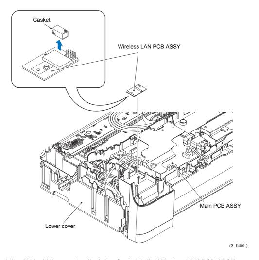
Assembling Note Make sure to attach the Gasket to the Wireless LAN PCB ASSY.
