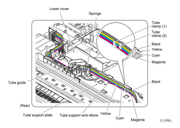
**Note** Bind the ink supply tubes with the two tube clamps. Bind magenta, cyan, and yellow together from the bottom with tube clamp (1). Bind black, yellow, and cyan from the top with tube clamp (2).
