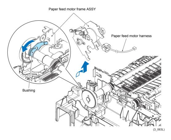
(4) Remove the two screws of the SCREW BIND M2.6x4 and remove the Paper feed motor from the Paper feed motor frame.
