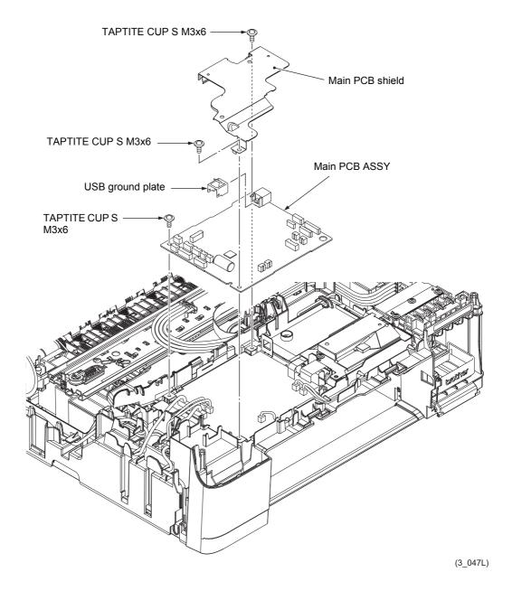
**Assembling Note** When the Main PCB ASSY is replaced, make adjustments by following Chapter 4 "1 IF YOU REPLACE THE MAIN PCB ASSY".
