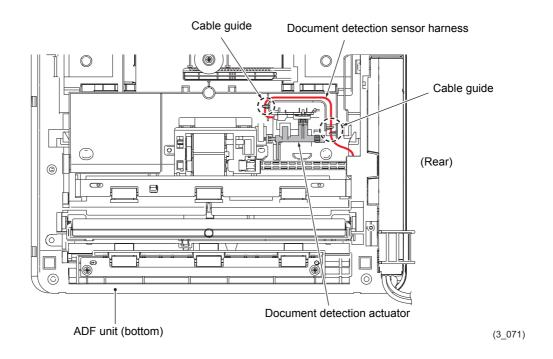
ADF unit top (only for models with ADF unit): ADF harness ASSY (ADF motor harness and ADF FG wire, Document detection sensor harness, Document scanning position sensor harness)
