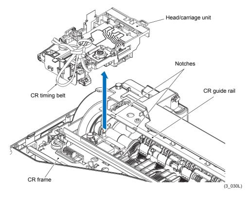
(22) Remove the CR timing belt from the Head/carriage unit.
