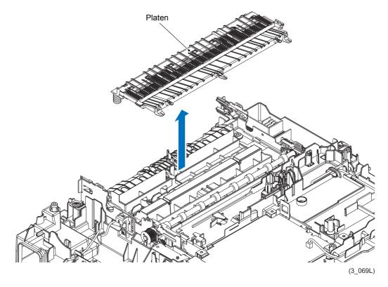
Assembling Note Make sure that the Platen springs are not folded or turned down.
