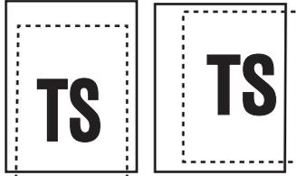
Scanning position failure
