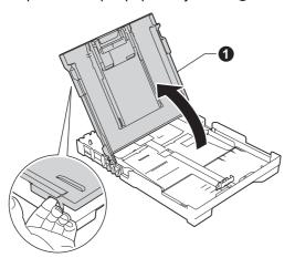
C Gently press and slide the paper width guides ● and then the paper length guide ② to fit the paper size.
