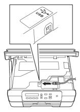
C Carefully guide the USB cable into the cable channel and out the back of the machine. Connect the cable to your computer.
