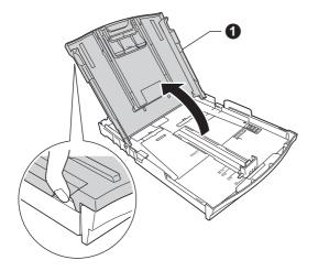
With both hands, gently press and slide the paper side guides • and then the paper length guide • to fit the paper size.
