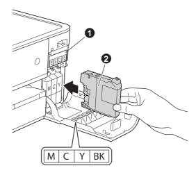
Gently push the back of the ink cartridge marked "PUSH" until the cartridge lever lifts. After all the ink cartridges are installed close the ink cartridge cover.
