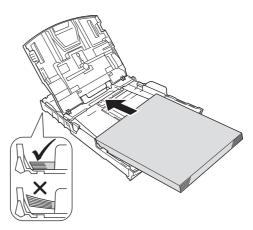
Gently adjust the paper side guides to the paper with both hands. Make sure that the paper side guides touch the edges of the paper.
