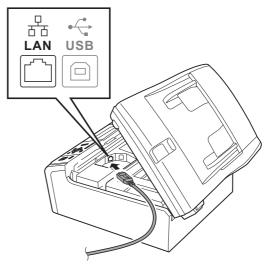
C Carefully guide the network cable through the trench as shown below, following the trench around and toward the back of the machine. Then, connect the cable to your network.
