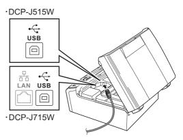
Carefully guide the USB cable through the trench as shown below, following the trench around and toward the back of the machine. Then connect the cable to your Macintosh.
