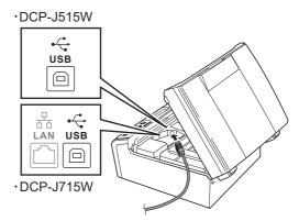
C Carefully guide the USB cable through the trench as shown below, following the trench around and toward the back of the machine. Then connect the cable to your computer.
