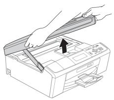
b Connect the USB cable to the USB socket marked with a 😽 symbol. You will find the USB socket inside the machine as shown below.
