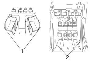
If you are not able to find the green protective part, DO NOT remove the ink cartridges before shipping. It is essential that the machine be shipped with either the green protective part or the ink cartridges in position. Shipping without them will cause damage to your machine and may void your warranty. 4 Lift the front of the machine and hook the long end (1) of the green protective part into the T-shaped hole underneath the machine. Push the forked end (2) onto the top of the paper tray.
