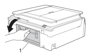
Clean the Paper Pick-up Rollers (1) with a soft lint-free cloth slightly moistened with water.
