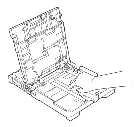
Olose the output paper tray cover and put the paper tray firmly back in the machine.
