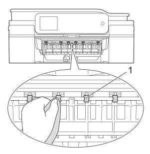
3 Lift the Jam Clear Flap (2), and then clean the back side of the Paper Feed Rollers (1) with a soft lint-free cloth slightly moistened with water.
