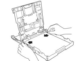
Fan the paper well and load it in the tray, and then adjust the paper guides.
