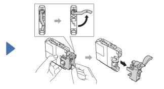
Follow the Touchscreen instructions to install the ink cartridges. The machine will prepare the ink tube system for printing.
