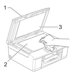
3 In the ADF unit, clean the white bar (1) and the glass strip (2) with a lint-free cloth moistened with a non-flammable glass cleaner.
