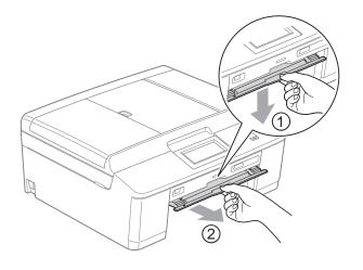
4 Using both hands, use the plastic tabs on both sides of the machine to lift the scanner cover (1) to the open position.
