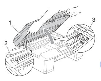
Move the print head (if necessary) to take out any paper remaining in this area. Make sure that jammed paper is not left in the corners of the machine (2) and (3).
