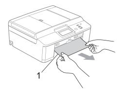
4 Lift the Jam Clear flap, and remove the jammed paper from the Disc Guide.
