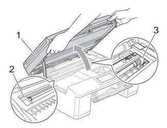
Move the print head (if necessary) to take out any paper remaining in this area. Make sure that jammed paper is not left in the corners of the machine (2) and (3).
