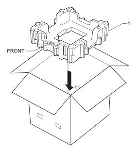
4 Wrap the machine in a plastic bag, then place it on the bottom packing material (1).
