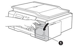
C Lift the cap of the ink tank for the colour you want to fill.
