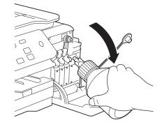
Push down on the cap of the ink tank to close it tightly.
