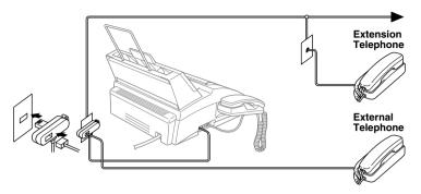
Whenever this external phone (or TAD) is in use, the screen displays **EXT. TEL IN USE**, and, if the fax handset is lifted, an alarm sounds.
