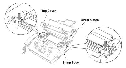
**3** Pull the jammed paper toward the back from the paper tray and remove it as per diagram A. If you can't, pull the jammed paper towards the front and remove it as per diagram B. If you cannot see any jammed paper, remove the ribbon cassette and check underneath. Remove any jammed paper.
