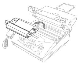
**4** To clean the machine's thermal print head, wipe the metal and plastic part with a lint-free cloth that is dry or lightly moistened with isopropyl alcohol as per diagram below.
