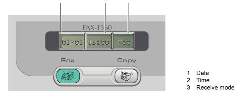
When the machine is idle (not being used) it will return to the default display shown above. The default display shows the date, time, and the current receive mode.
