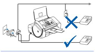
Set the receive mode to 'External TAD' for FAX-1355 and FAX-1360, or 'Manual' for FAX-1460 if you have an external answering machine. For details, see Connecting an external TAD (telephone answering device) in Chapter 7 of the User's Guide.
