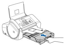
While holding the paper tray in place, pull out the paper support ( ① ) until it clicks and unfold the paper support flap ( ② ).
