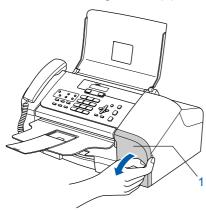
3 Pull the lock release lever down and remove the yellow protective part (1).
