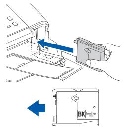
7 Lift the lock release lever and gently push until it clicks, and then close the ink cartridge cover.
