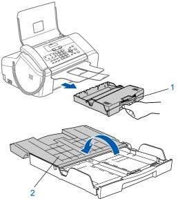
Press and hold the universal guide release button (1) as you slide out the front of the paper tray to match the paper size you are using.
