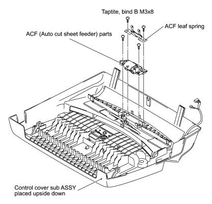
(3) Disassemble the ACF parts as illustrated below.
