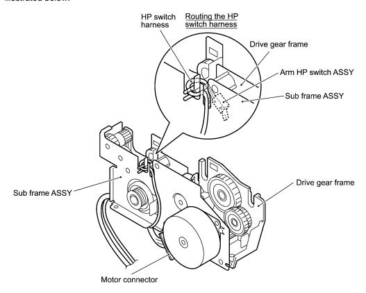
• Route the motor harness (or motor flat cable) and HP switch harness along the guides on the bottom of the drive unit.
