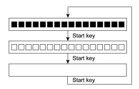
(3) Press the **Stop** key in any process of the above pattern cycle. The equipment beeps for one second and returns to the initial stage of the maintenance mode.
