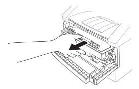
3 Pull the toner cartridge out of the drum unit assembly while holding down the lock lever with your right hand. For more information, see "Replacing the Toner Cartridge" in this chapter.
