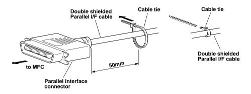
2 Attach the Filter core, pressing until you hear a click, between the Parallel Interface connector and the Cable tie.
