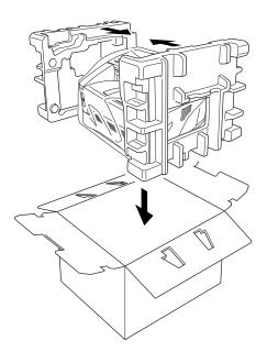
**7** Place documents (manual and printed material) and the cables (MFC-9650), document tray and document support, drum unit and toner cartridge assembly into the carton as shown below.
