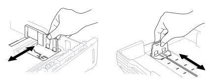
3 Fan the paper well. Load paper in the paper cassette. Press down on the paper to flatten it in all four corners, keeping the paper level below the guide. The cassette can hold up to 250 sheets of 20 lb (75 g/m²) paper.
