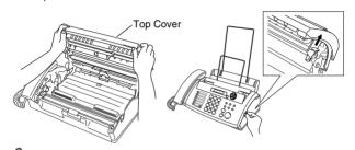
3 Pull the jammed paper gently from the paper feeder toward the front of the fax machine as per diagram A.
