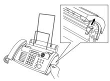
Remove the print cartridge containing the used ribbon and set it upside-down with the blue gear in the upper left corner.
