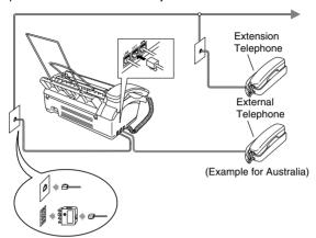
Whenever this phone (or TAD) is in use, the LCD shows EXT. TEL IN USE and, if the fax handset is lifted, an alarm sounds.
