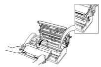
To clean your fax machine's print head, wipe the print head with a lint-free cloth that is dry or lightly moistened with isopropyl alcohol.
