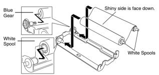
Insert the teeth of the white spool into the cutouts of the cardboard core.
