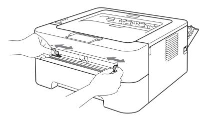
5 Using both hands, put one full sheet of labels or one envelope in the manual feed slot until the front edge touches the paper feed roller. When you feel the machine pull it in, let go.
