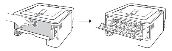
Pull down the tabs at the left and right hand sides to open the fuser cover (1).
