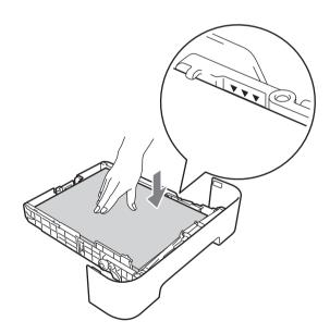
4 Put the paper tray firmly back in the machine. Make sure that it is completely inserted into the machine.
