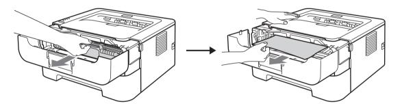
If you cannot remove the drum unit and toner cartridge assembly easily, do not use extra force. Instead, go to step 4.
