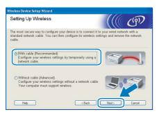
9 For configuration, you must temporarily connect your Brother wireless device (your printer) directly to a free port on your access point, hub or router using a network cable. When the following screen appears, insert the network cable to the access point and then to the printer. Click Next.
